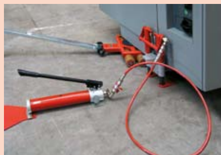
Application with „Primus“ and central pump
