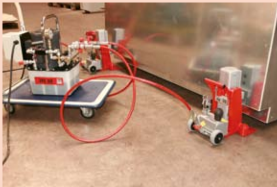
Electric pump JPE 30-NVR with 2 jacks in operation
